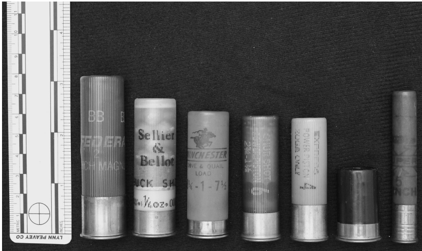
Figure 2.3 (See color insert.) A cross-section of various size shot shells, from left to right: 12-gauge 3½" Super Magnum, 12-gauge 3" Magnum, 12-gauge 2¾", 16-gauge 2¾", 20-gauge 2¾", Aguila 12-gauge 1½", and .410 3" shell. (Images from author's collection.)
